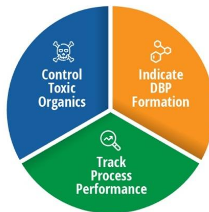
Figure 1: Three principal roles of TOC monitoring in potable reuse.
